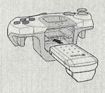
The Jump Pack should always be inserted into Expansion Socket 2. \*When the Jump Pack is inserted into Expansion Socket 1 of the Sega Dreamcast Controller, the Jump Pack connects, but does not lock. If the controller is jarred, the Jump Pack may fall out during game play or otherwise inhibit game operation.
